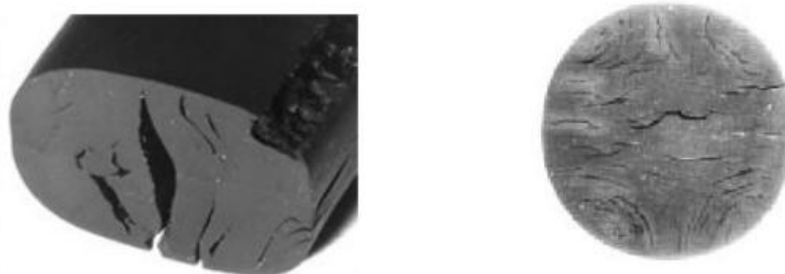
Figure 1: Samples with Fractures caused due to Rapid Gas Decompressions (RGD)
