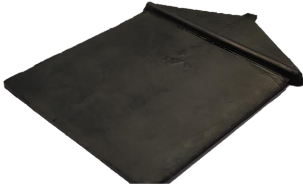
Figure 8: Injection moulded plate with visible impurities [Image: IKV]
