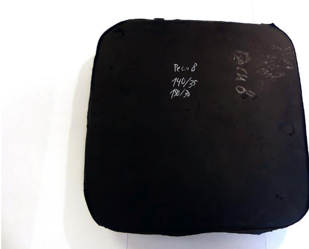
Figure 10: Final block of PECU-H foam [Image: Köpp]
